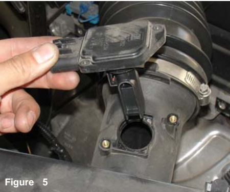
Figure 2 Depress the locking clip and remove the electrical sensor harness from the mass air flow sensor.
