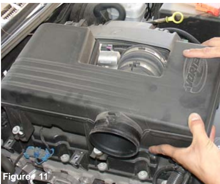
Figure 8 Remove the two screws that secure the resonator box to the throttle body and mounting brackets.
