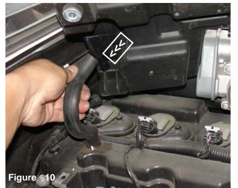
Figure 7 Once the intake tube has been removed from the resonator inlet (A) continue to pull the entire air intake and air box cleaner assembly from the resonator box (B).
