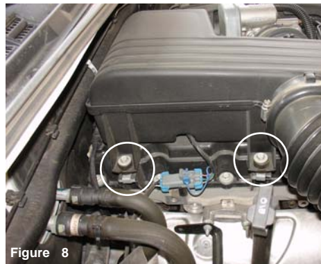
Figure 5 Once the screws have been removed, continue to remove the mass air flow sensor from the sensor housing.
