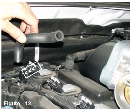
Figure 9 Loosen the hose clamp that is connected to the throttle body as shown above.
