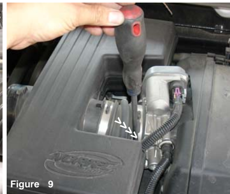
Figure 6 Loosen the clamp on the resonator inlet that connects the stock intake tube to the resonator. Remove the intake tube from the resonator.
