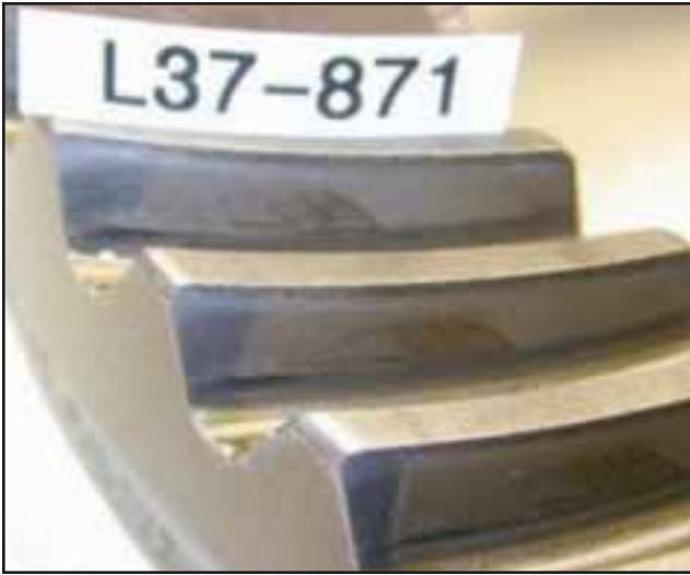
Ring gear exhibits very low wear.
